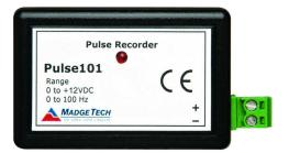
The Pulse101 is a miniature, low-cost recording device which senses pulse inputs or contact closures from external sources such as transducers and/or pulse initiators. It can collect as many as 100 pulses per second and store up to 16,383 totalized pulse counts in its non-volatile memory. Start and stop the device directly from a computer and its small size allows it to fit almost anywhere.
